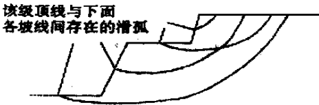
图 6 坡脚两边均搜索一安全系数最小的圆弧 Fig. 6 Arcs with the minimum safe factor beside slope feet
